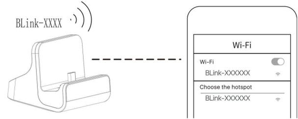
After connected, it is normal when you get a message like 'no internet available, unsecured network' etc. It is OK as long as camera is connected with "BLink-XXXX" WIFI LAN.
